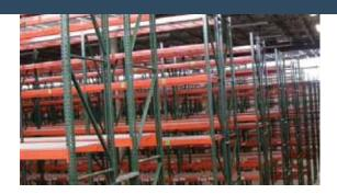
**Three-Point Safety Catch** — Each beam has 3 rugged studs (4 on heavy-duty) that engage the tapered keyhole slots in the upright with a compression fit. Integral safety lock automatically locks into place when beam is properly seated.
