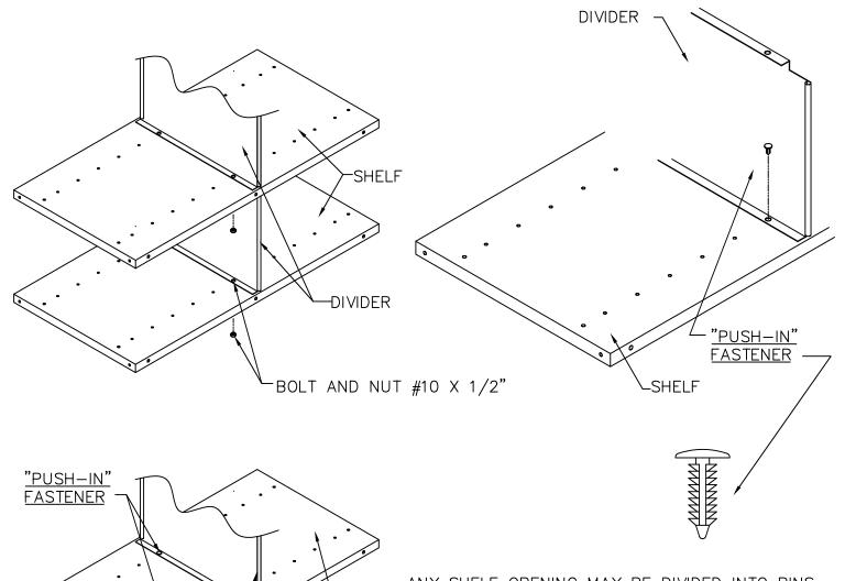
ANY SHELF OPENING MAY BE DIVIDED INTO BINS BY THE INTSALLATION OF DIVIDERS. TO INSTALL DIVIDERS, PLACE THEM IN POSITION BETWEEN THE SHELVES AND ALIGN THE HOLES IN THE DIVIDER FLANGES WITH THE HOLES IN THE SHELVES. ATTACH THE DIVIDERS TO THE SHELVES WITH "PUSH—IN" FASTENERS AS ILLUSTRATED.
