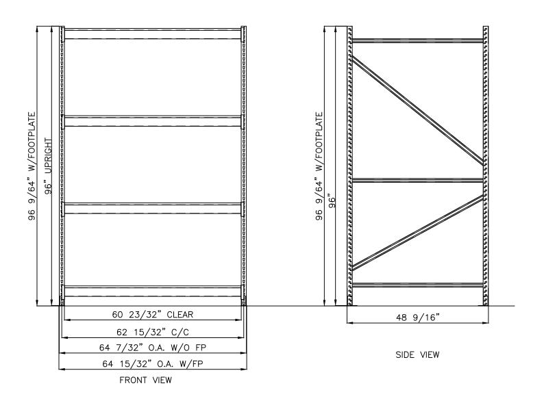
60"W X 48"D X 96"H BULK STORAGE RACK WITHOUT DECKING
