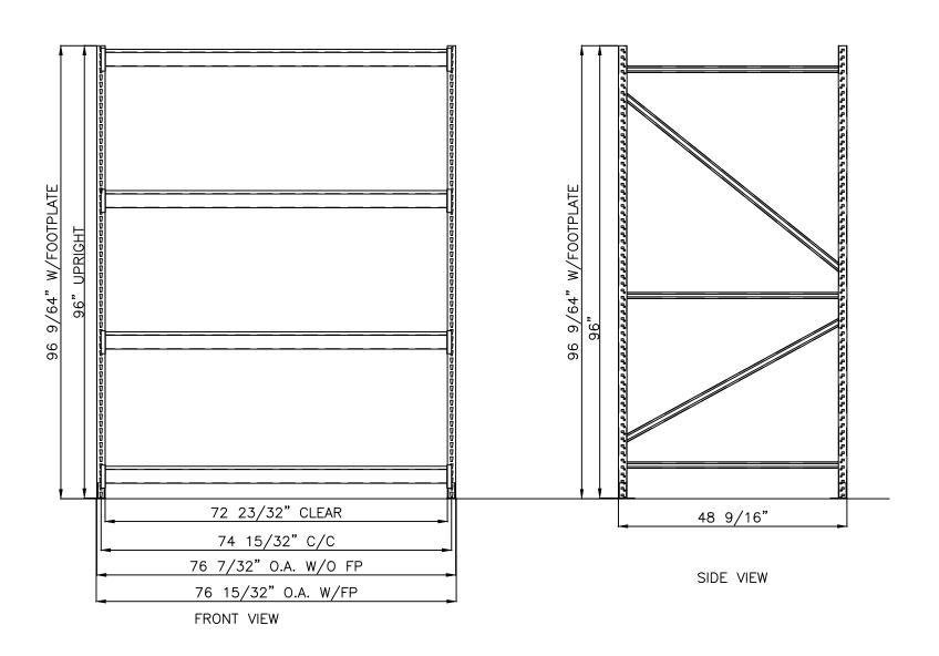
72"W X 48"D X 96"H BULK STORAGE RACK WITHOUT DECKING
