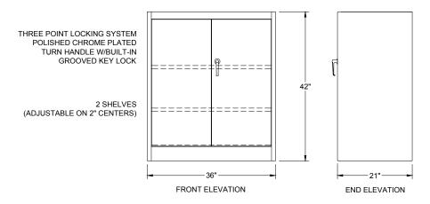
LYON 1000 SERIES STORAGE CABINET CAT# 1040 SET-UP UNIT 36"W x 21"D x 42"H COLOR: \_\_\_\_\_
