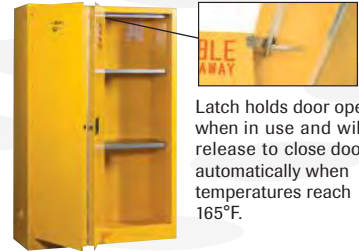
Self-closing doors feature manual latch with fusible link.
