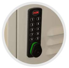
Digital locks features a slimline electronic lock. A user provides their own 4-digit code to secure their items. Once the code is re-entered to unlock the door, the lock re-sets for the next user. The colored indicator ring of the pop-out handle shows at a glance if the locker in use or available. Each lock uses 2 AA batteries. One master key is included per order.
