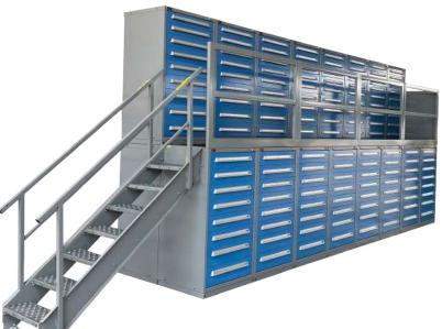
A standard system begins with two rows of stacked modular drawer cabinets, stairs, handrails and a heavy-duty mat that is placed over the lower row of cabinets to create a walkway.
