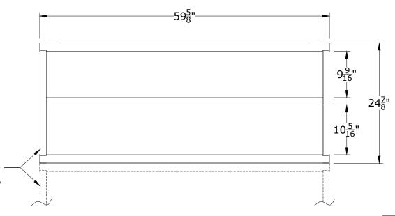
OVERHEAD CABINET WIDTH MUST MATCH WIDTH OF LOWER CABINET. DOUBLE OVERHEAD CABINETS CAN BE ASSEMBLED OVER TWO (2) STANDARD 30W CABINETS. FIELD INSTALLATION ONLY. THIS WILL PRODUCE A 3/8" GAP ON EITHER SIDE OF THE OVERHEAD UNIT.
