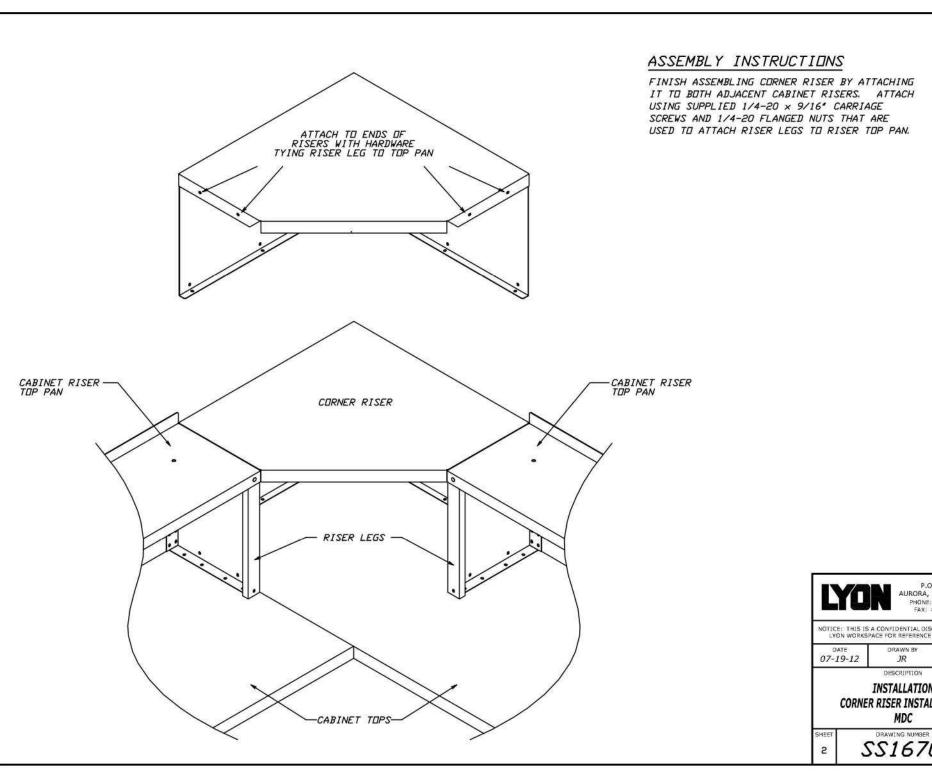
FINISH ASSEMBLING CORNER RISER BY ATTACHING IT TO BOTH ADJACENT CABINET RISERS. ATTACH SCREWS AND 1/4-20 FLANGED NUTS THAT ARE
