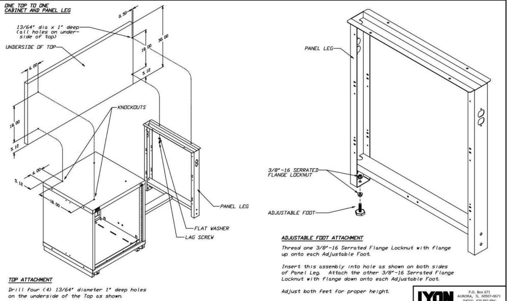
Punch Knockouts as shown in top of cabinet and remove sufficient top drawers and carriers and mark for reinstallation.
