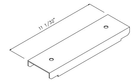
NOTE: ORDER CAT#9252 WHEN USING #9246 OR #9247 GRATING, WHEN EXTRA ARE REQ.'D WITH #9282,#9283 OR 9284 GRATING OR USE WITH#9251 GRATING SPLICER WHEN SPLICE DOES NOT FALL ON A SUPPORT
